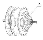
Place the bushing and stop pin onto the motor axle from the left side. Insert the motor into the rear fork end.
