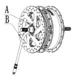
Install the freewheel onto the motor axle from the right side. Tighten it with socket and adjustable wrench. [35 N.m]
