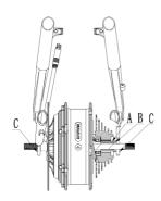
Place two 4mm bushings onto the motor axle from the right side. Place a M12 flange nut, and tighten it with 19mm wrench. Install the cap nut. [40-45 N.m]
