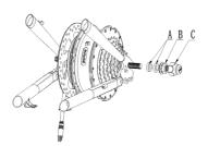
5. Place the stop pin onto the motor axle from the left side. Place a M12 flange nut, and tighten it with 19mm wrench. Install the cap nut. [40-45 N.m]
